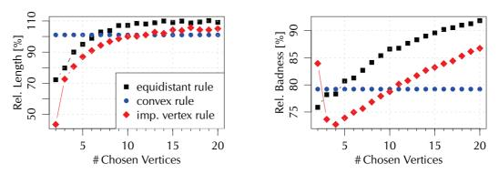
**Figure 7.9.** Evaluating the effect of the smoothening rules on GF. We report the relative amount by which the route's length (left) and badness (right) change while varying the number of vertices the algorithm selects to compute shortest paths (cf. Section 7.2.1). The key of the left figure also applies to the right.
